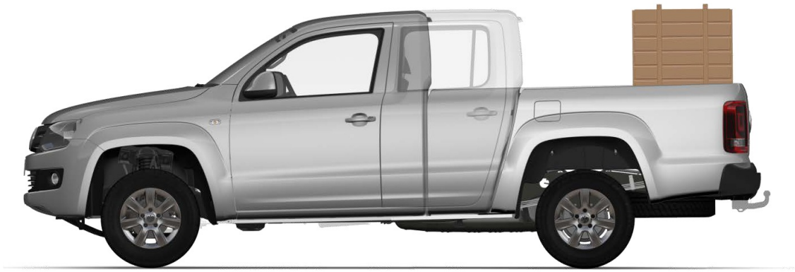
Fig. 2: One-sided weight distribution (side view)
